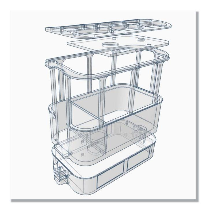
The 2mm acrylic piece fits snugly onto the inner of the main body and represents the top of the tanks. Tank fillers are supplied, along with a chimney and sand-dome.
