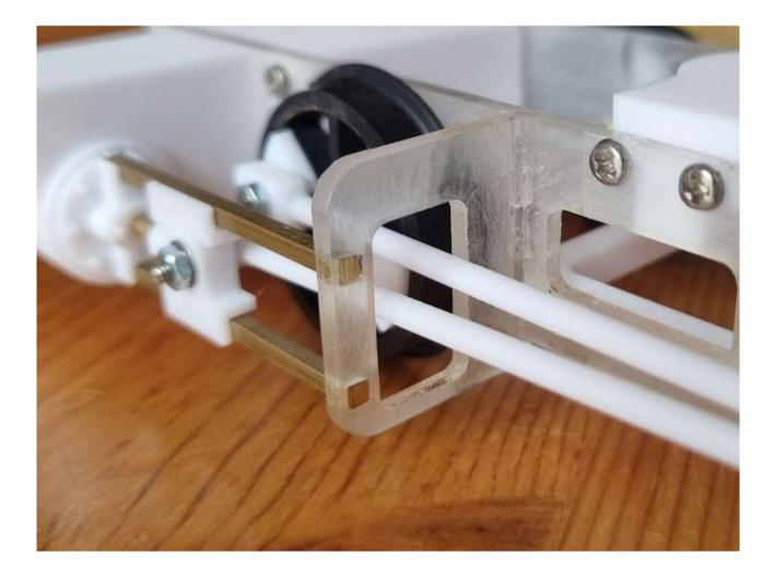
Locate the cylinder block relevant to the frame and attach using two 8mm M2 screws. I have designed most of the chassis to accept the 8mm M2 screws as self-taping, some of the holes may require opening slightly to get the screw started.
