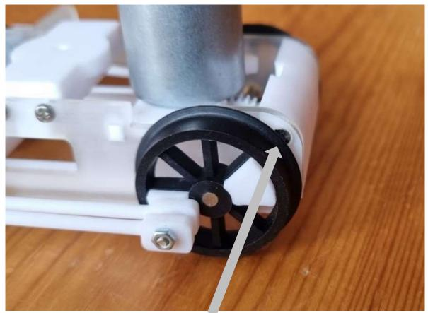
The rear stretcher screw (conehead) countersunk into the acrylic to allow rear wheelset clearance
