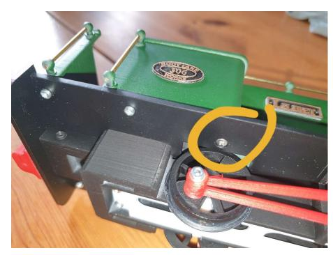
The footplate will require two holes to be countersunk. The two foremost holes that attach the leading edges of the bunkers will need countersinking to accept the two 10mm conehead M2 screws.
