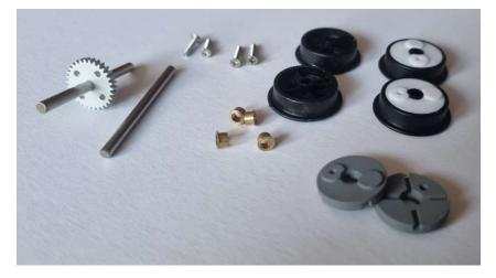
The two inserts lower right are in grey undercoat, while the other two are still white filament. These last two have been pressed into the Binnie wheels.
