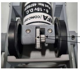
Locate the two gearbox parts. (Photo is VARSITY, but the gearbox is the same on WILLIAM)
