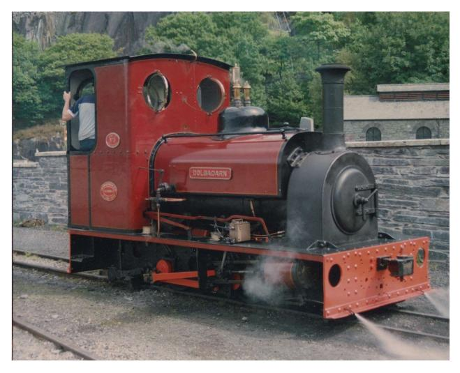
DOLBADARN at the Llanberis Lake Railway. Note that the locomotive has lost its sand-pots and retained the shortened chimney from her time in the quarries when the cab was also removed!
