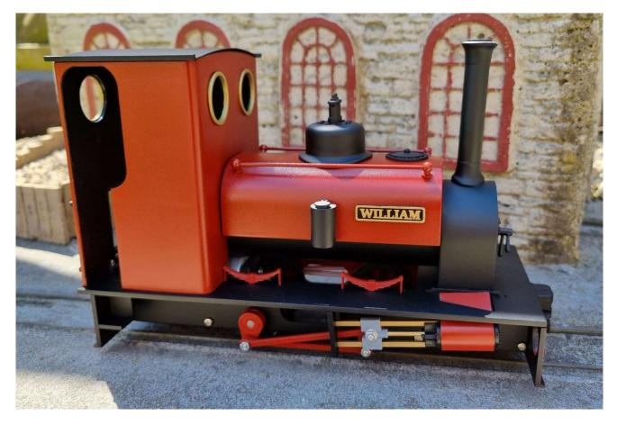
Other details include chimney (there are two, a long & a short), dome, sandpots, tank filler, firedoor, regulator, reverser & gauge glasses, smokebox door & dart.
