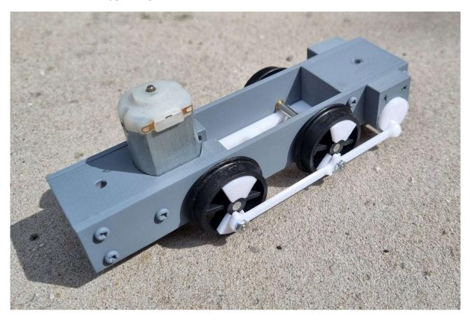
This image also shows the motor and the dummy Jackshaft & rods.
