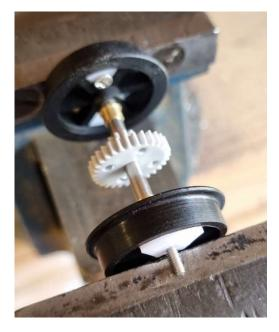
Keeping the whole wheelset square to the axles and using the jaws of the vice against the inserts, squeeze the wheels onto the axles. Notice the brass bushes. Also, both crankpins are currently in line.
