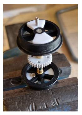
With the wheelsets quartered, they can be added to the chassis unit. Drop the wheelsets in, the front wheelset is the driven set, so will be the one with the grey gear.
