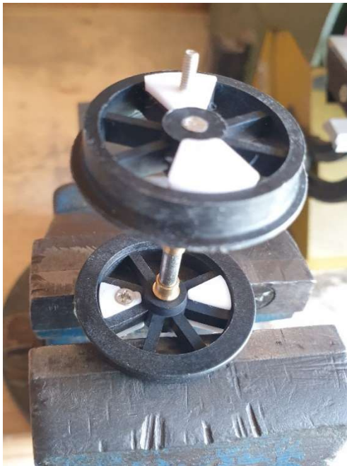
Image is of a loco wheelset (note the longer crankpins on one wheelset, not relevant to the "Nō 6" chassis)
