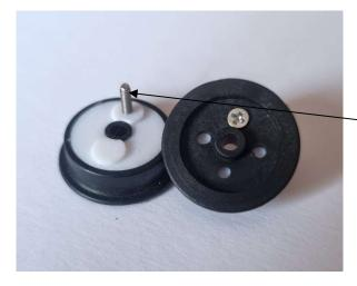
Using a vice, press the wheel inserts into the Binnie wheels.
