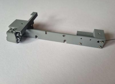
Now take the front & rear stretchers and using a further six M2 screws, attach the stretchers to the two stretchers to the frame-plate.
