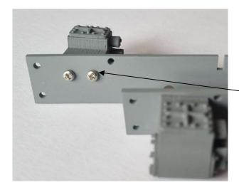
Take one of the cylinder blocks and a frame and attach the block to the frame through the two holes at the front of the frame using two of the M2 panhead screws.
